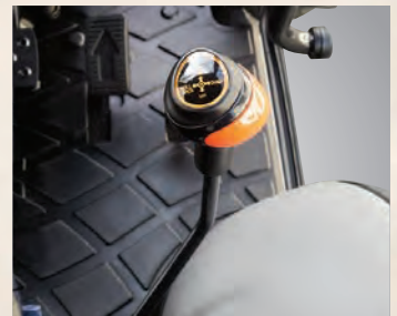
FRONT LOADER CONTROL LEVER
